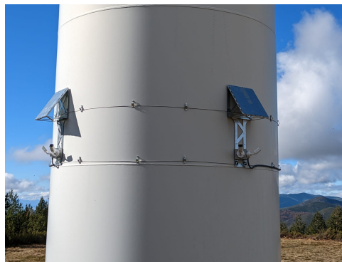
Figure 7: 4K camera with anti ice roof
