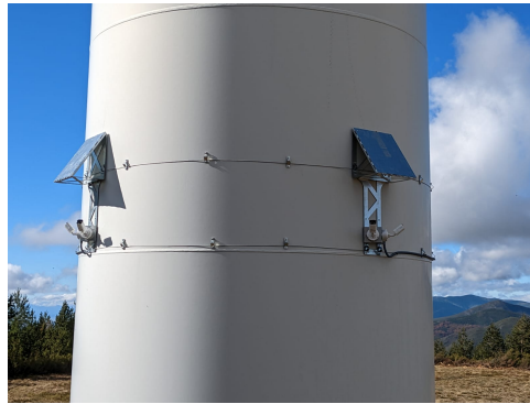
Figure 7: 4K camera with anti ice roof
