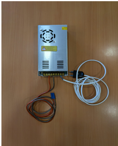
Figure 4: 220V to 48V converter
